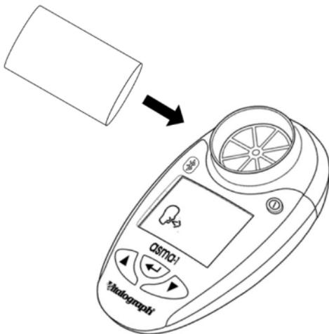
*Figure 2. Mouthpiece inserted into flowhead*
