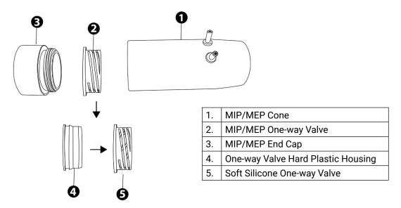
Fig 2: Disassembled MIP or MEP Flowhead
