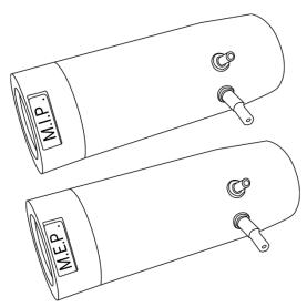
Fig 1: MIP and MEP Flowhead Assemblies Complete
