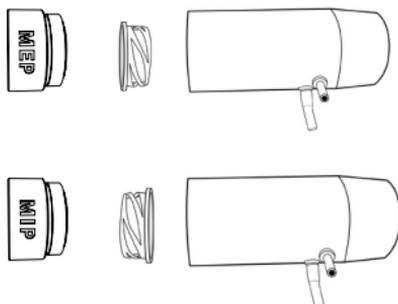
Figure 5: Orientation of one-way valve
