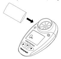
Figure 2. Mouthpiece inserted into flowhead
