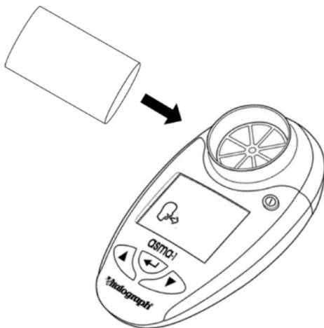
Figure 2. Mouthpiece inserted into flowhead
