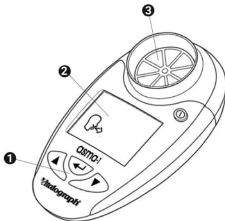
Figure 1 Vitalograph asma-1 Components
