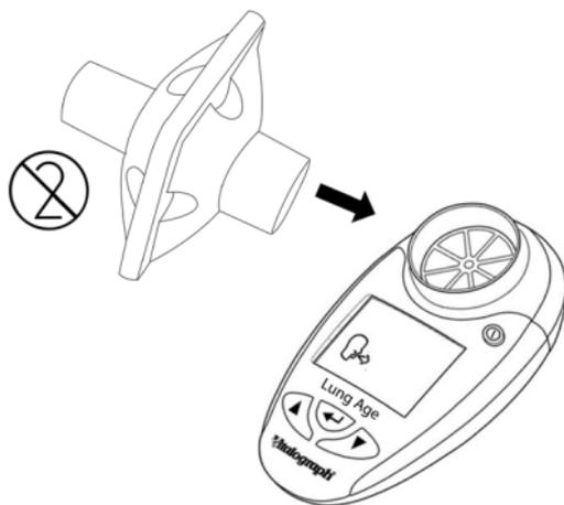
*Figure 2. Mouthpiece inserted into flowhead*
